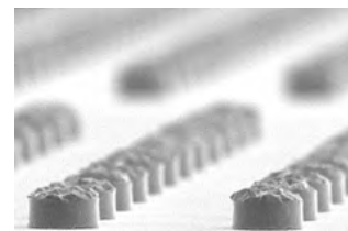
Micro-bumps formed with 50 µm thick JSR THB-151N negative resist
