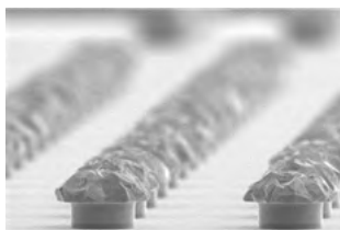
Bumps formed with 20 µm thick JSR THB-126N negative resist
