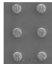
Micro-bumps formed with 50 µm thick JSR THB-151N negative resist
