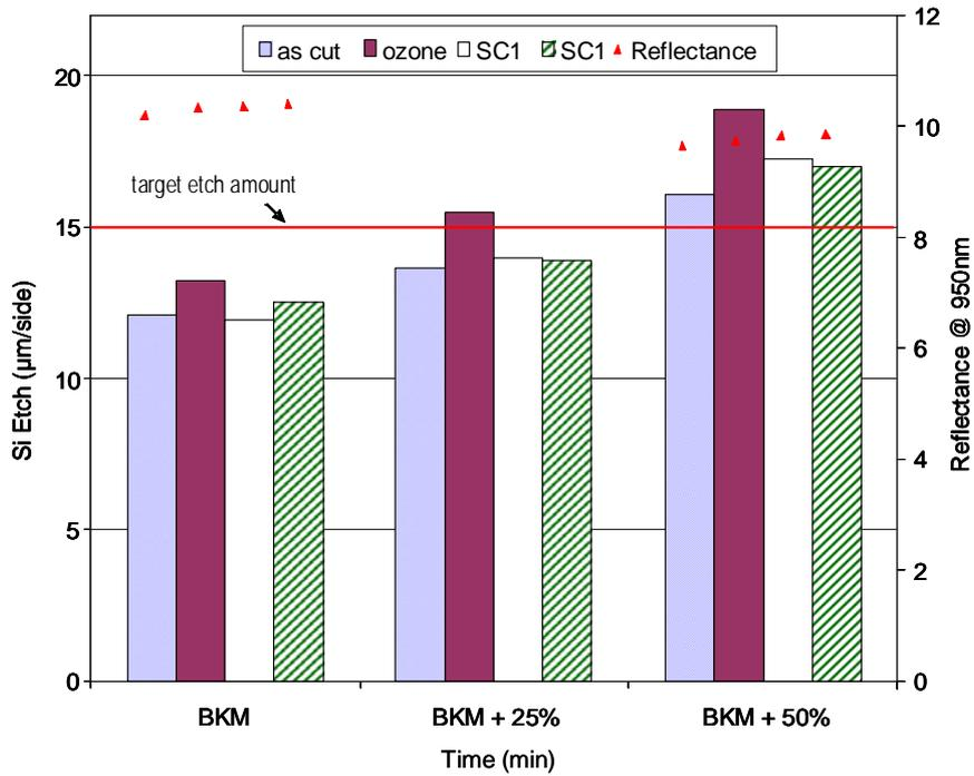
Figure 1: Si etch and reflectance versus various pre-clean processes.
