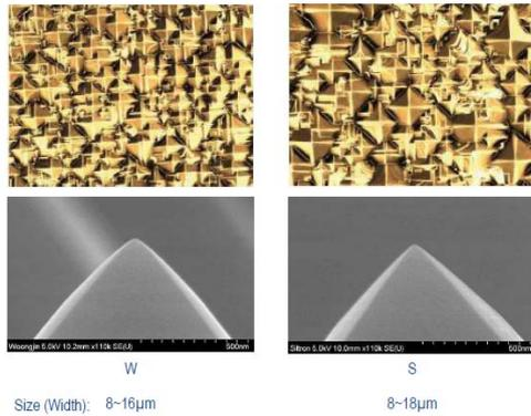
Figure 2: pyramid patterns after standard KOH/IPA texturization for different wafer types (slurry and diamond-cut).
