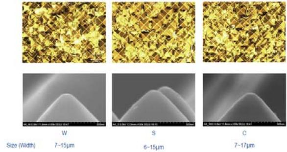
Figure 3: pyramid patterns after standard KOH/IPA texturization for different wafer types (slurry and diamond-cut).
