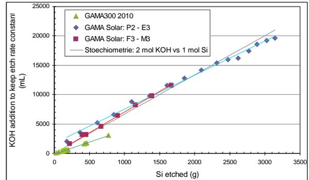
Figure 3: Volumes of KOH required to etch Si in production is in agreement with theory.
