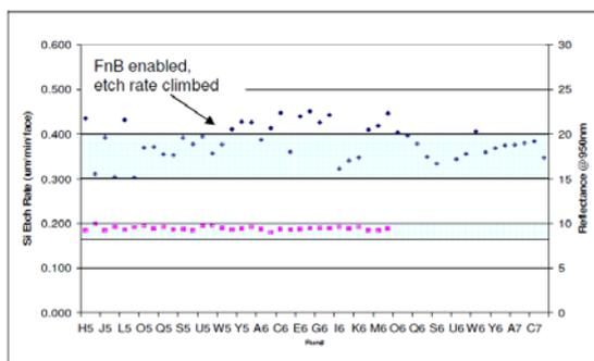
Figure 6: Etch rate (ER) and reflectance over time with dynamic feed/bleed and ICE controls.
