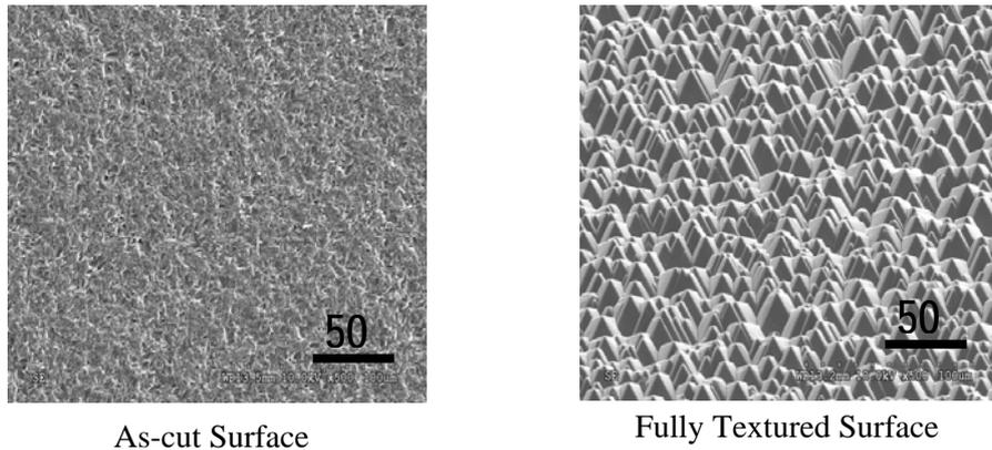
Figure 1: A Sample of surface texturization
