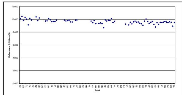
Figure 5: Reflectance of texturized wafers vs. multiple process lots.
