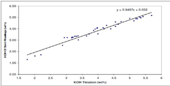
Figure 2: Measured and predicted concentrations of KOH.
