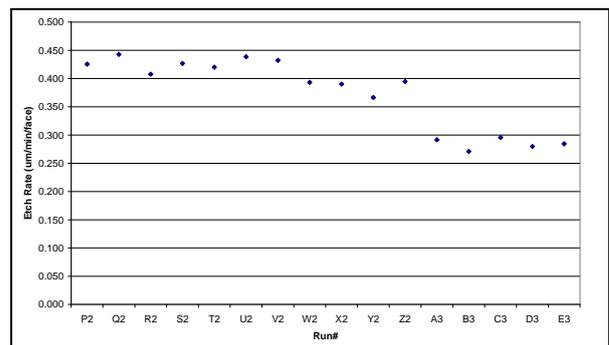
Figure 7: Etch rate (ER) over time without dynamic feed/bleed and ICE controls.
