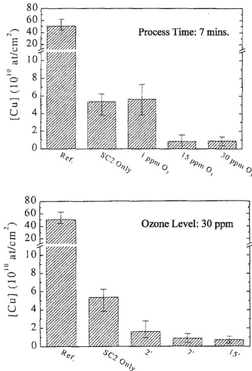
Figure 6. Cu removal by 1:1:5 SC2 at 65°C versus DI-O<sub>3</sub> water with various dip time and ozone concentration; (Top) effect of ozone level and (Bottom) effect of dip time. (Ref. 21)
