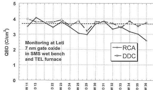
Figure 8. Monitoring results obtained between RCA and DDC cleanings performed in parallel on the same wet bench, followed by alternative dry and wet gate oxidation processes. (Ref. 10)
