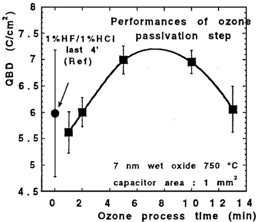
Figure 2. Comparison of QBD performance for samples receiving HF-last and DI-O<sub>3</sub> water treatments. (Ref. 9)
