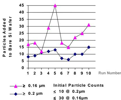
Figure 12. Particle counts on bare Si surfaces after the DIW/O<sub>3</sub> resist stripping process. (Ref. 35)
