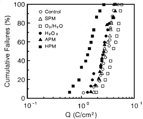
Figure 3. Cumulative failure characteristics of MOS diodes negatively biased with constant current density, which contained 6 nm gate oxide incorporating chemical oxides formed by various chemicals. (Ref. 7)
