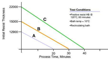
Figure 11. Etch rates in DIW/O<sub>3</sub> processing for different types of photoresist (A: AZ1518, B: HIPR6512, C: Shibley SPR2). (Ref. 35)
