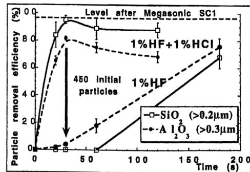
Figure 7. Particle removal efficiency of SiO<sub>2</sub> and Al<sub>2</sub>O<sub>3</sub> by 10-minute DIW-O<sub>3</sub> (3 ppm) rinse followed by diluted HF/HCl or HF dip. (Refs. 9,20)
